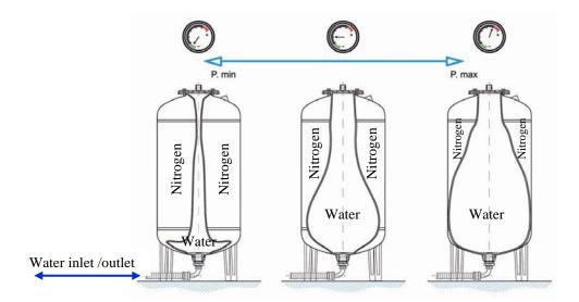
When the maximum required pressure is reached (pump stop pressure), the pressure switch cuts off the flow of water between the pump and AMR-*Plus* Inox hydropneumatic tank. At this moment there will be a volume of water stored inside of the hydropneumatic tank at a pressure equal to the stopping pressure of the pump.
